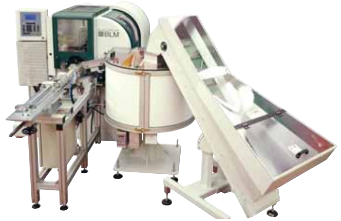
AST80 + AL38 + VIBRATING BOWL FEEDER
